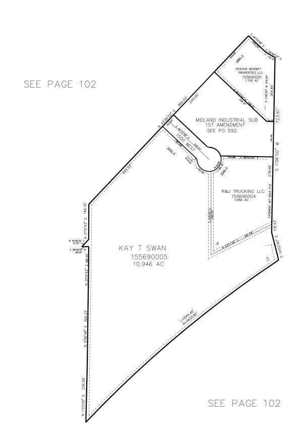
10' UTILITY & DRAINAGE EASEMENTS EACH SIDE OF PROPERTY LINES AS INDICATED BY DASHED LINES EXCEPT AS OTHERWISE SHOWN.
